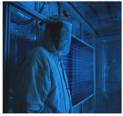
2. UV-irradiation of 200W/m² in humid environment in a climatic cabinet
