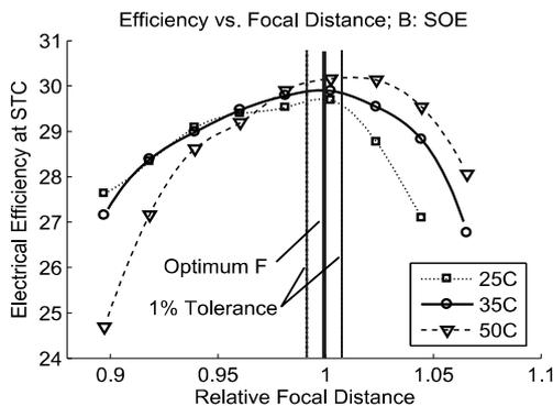
**FIGURE 4.** Efficiency curves for the Martifer optical system with optimal focal distance and 1% tolerance band.
