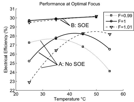
**FIGURE 5.** Temperature sensitive for systems operating at their nominal focal distance
