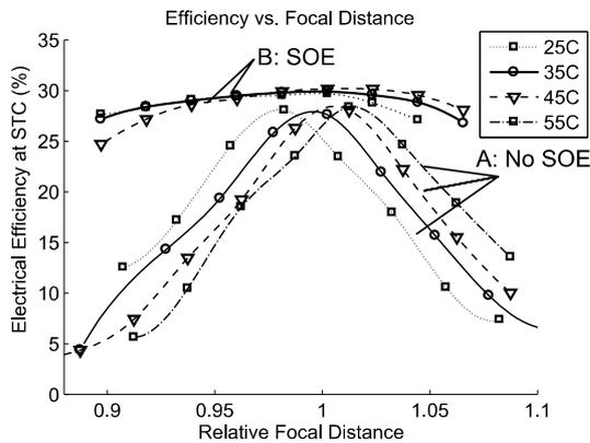
**FIGURE 3.** Comparison of focal distance vs. efficiency curves at different temperatures for the two systems.
