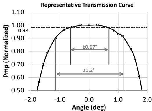
FIGURE 8. The representative module level transmission curve (rotated about module long axis) as measured in solar simulator, displaying a very flat curve.
