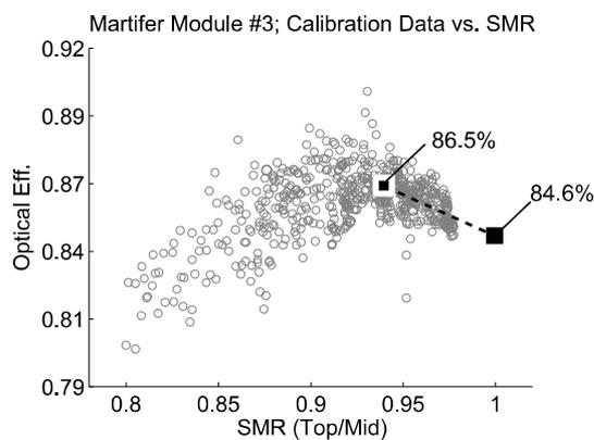
FIGURE 7. Effective optical efficiencies measured outdoors.
